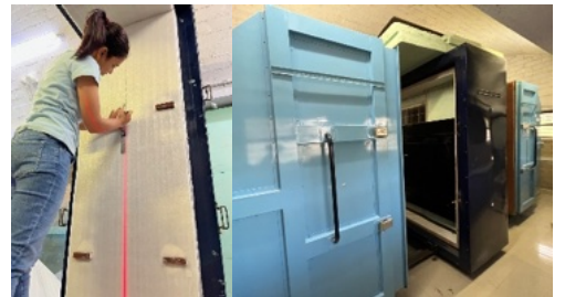
Figure 3 Hotbox Setup for moisture buffering testing
