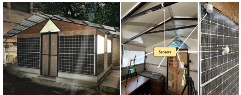
Figure 4 Setup for data collection for calibrating simulation model of E-O-L BIPV at IISc
