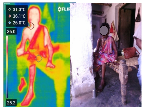
Figure 5 On-field Occupant comfort data ; Thermal Image (Left), corresponding to regular camera image (Right)
